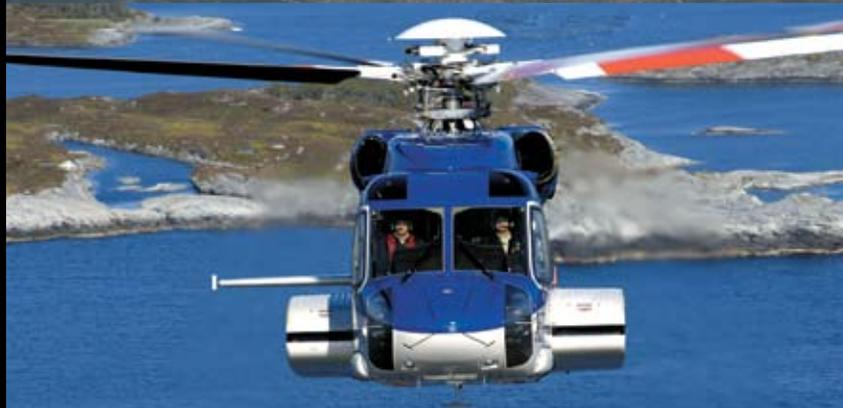
One of our newest technologies, the Rotor Ice Protection System (RIPS), senses and removes icy build-up on helicopter blades to enable flight during known icing conditions. Using this system, Sikorsky's S-92 helicopter was the first to be certified by the Federal Aviation Administration (FAA) for all-weather flight safety standards. Without this technology, the helicopters would be grounded during icy weather conditions.
