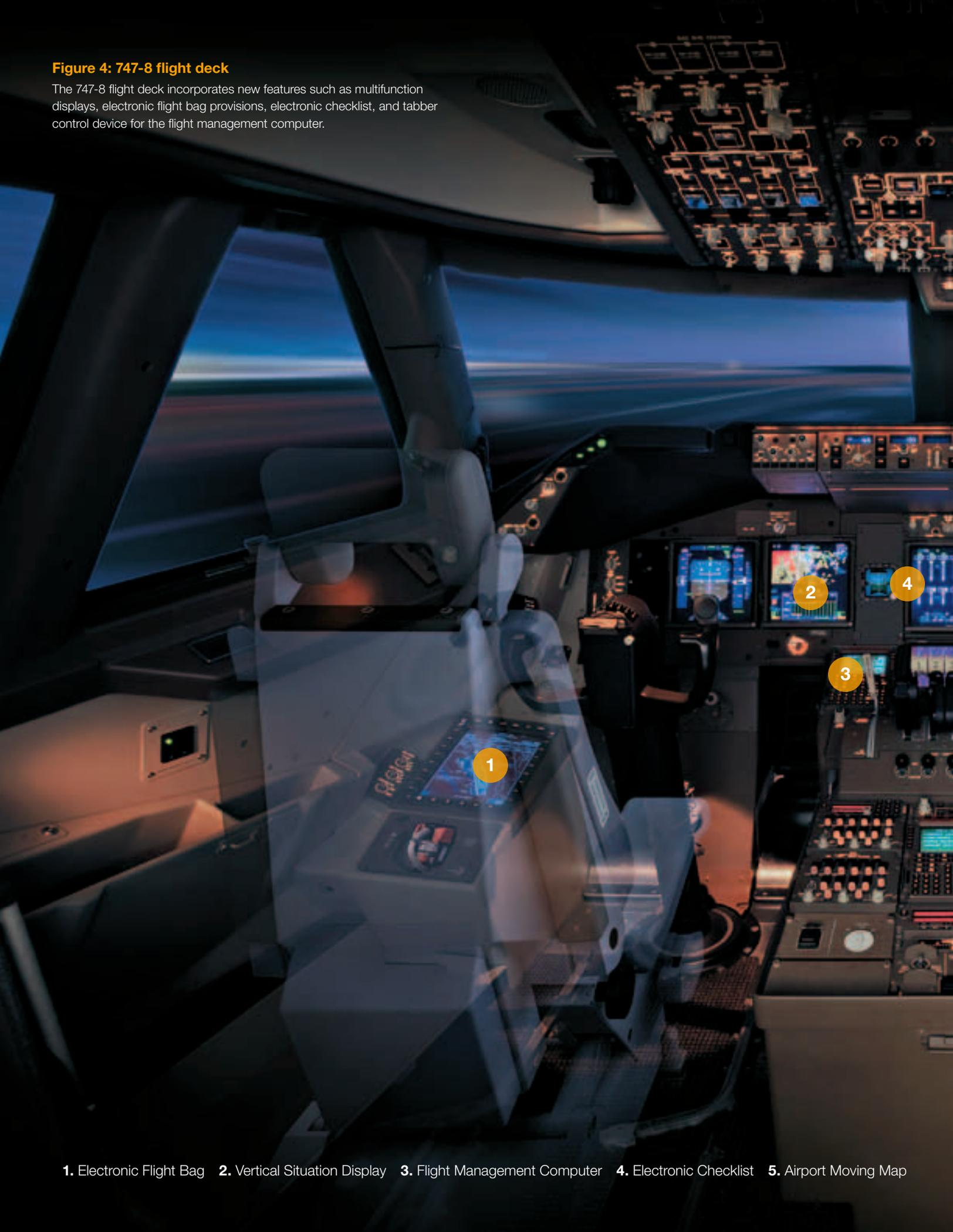
1. Electronic Flight Bag 2. Vertical Situation Display 3. Flight Management Computer 4. Electronic Checklist 5. Airport Moving Map
